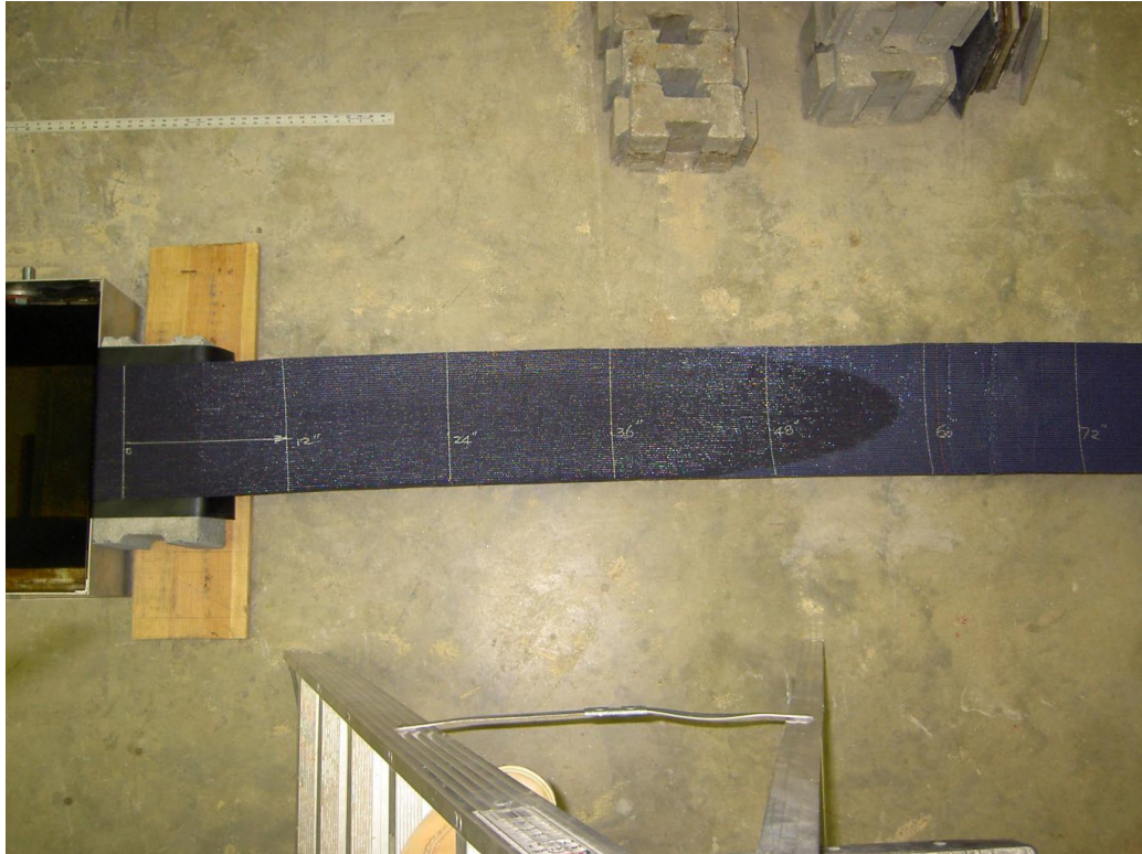
Figure 2.2 Water Movement in Fabric at Zero Hydraulic Gradient
