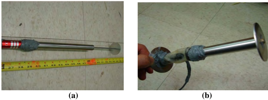
FIG. 2. Instrumentation sensors for the test lane sections: (a) LVDT; (b) customized potentiometer
