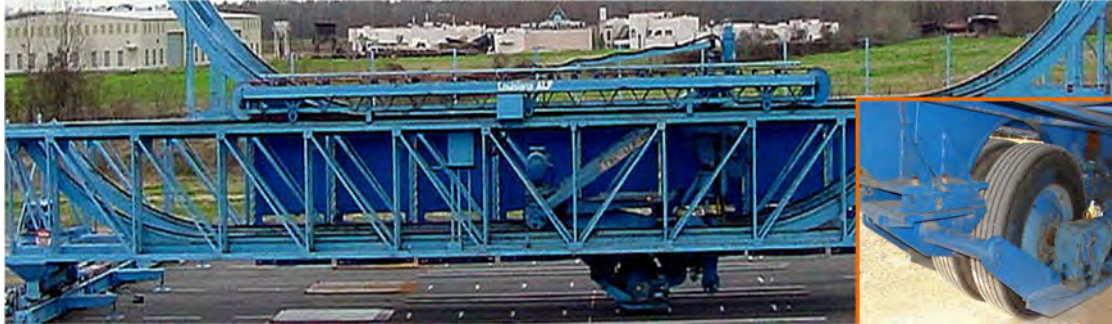
FIG. 3. The accelerated load facility (ALF) with an insert of the dual-wheel assembly.
