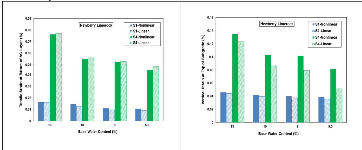
**Figure 5. Horizontal Tensile Strain at Bottom of AC for Structures 1 and 4**
